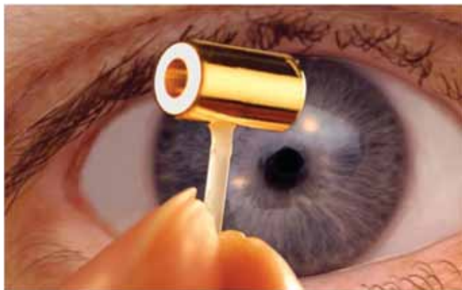
Figure 5. A closeup view of a fusion-fuel-filled spherical capsule known as a holhraum, the German word for “cavity.”
